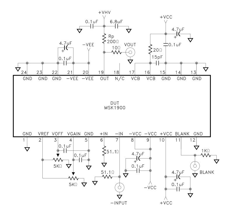
The connections shown above are for the MSK 1900 evaluation board. + Vcc should be connected to VCB through a  $20\Omega$  resister with a 15pF capacitor to ground. This will help to filter power supply noise and provide a stable voltage at VCB. RP is an external component and must not be located near ground planes if possible. A high quality resistor such as Bradford Electronics P/N FP10-200 is required for optimum response times.
