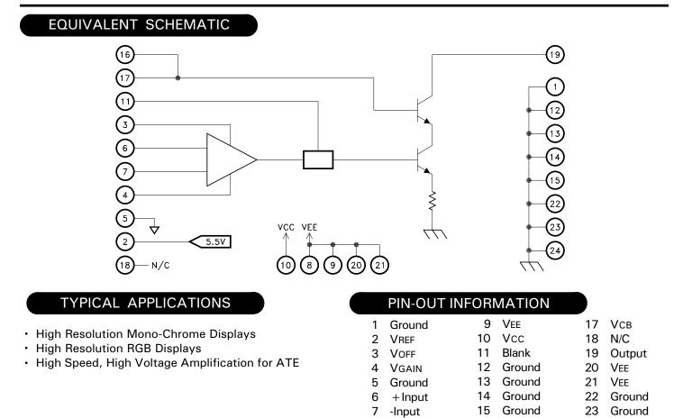
NOTE: All pins must be connected for proper operation if labeled.
